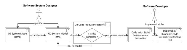
Figure 2.2: The main workflow with O2 for creating software systems.
