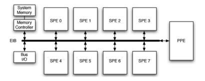
Figure 1: Cell BE Architecture
