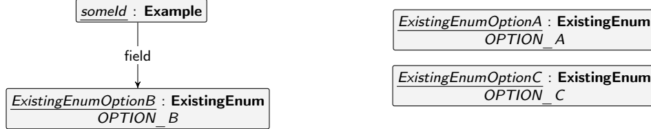
(c) IG_{EnumFieldFlags} with one node and its edge referencing enumeration option OPTION\_B
